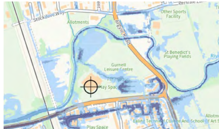
Extent of Flooding from Surface Water (Environment Agency)
